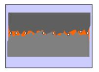
The film resistance is the resistance caused by materials deposited on to the contact during manufacture and later during the life of the relay. This will leave a very thin layer of an insulating 'goo' across the face of the contact rivet. The smoother the contact surface, the less the insulating layer will be but, of course, it is impossible to make a perfectly smooth surface.
